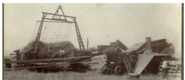
A wagon is unloaded using a huge net, and grain is pitchforked to a conveyor belt on a steam driven thresher and separator. Steam engine is out of picture at left, turning the conveyor belt in foreground. Sacks filled with grain are stacked at far right. Williams photo 1964-17
